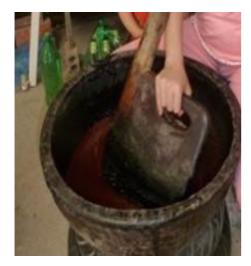
Figure 3-4 Heating and Stirring the Lacquer to Mature it, [Photograph] Thomson, E.
