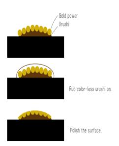
Figure 3-17 Diagram of Takamaki-e Technique by Sugano, Kaori (s.d.). At: http://suganokaori.com/tec.e.html (Accessed on 12.02.2016)
