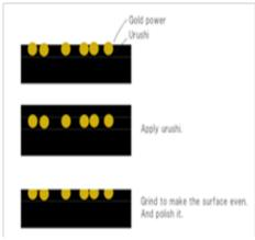
Figure 3-16 Diagram of Togidashi maki-e technique by Sugano, Kaori (s.d.) At: http://suganokaori.com/tec.e.html (Accessed on 12.02.2016
